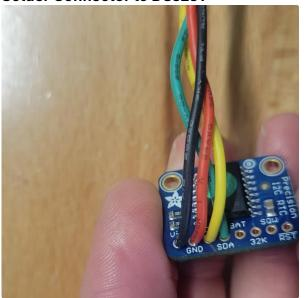
Although I added a plug here, you could just cut the Heltec supplied wire and solder directly to the DS3231.
