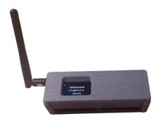
Adding a ChatterBox node to your cluster will provide additional range and resilience to all devices in your cluster. This is also the device I personally add larger antennas and amplifiers to, with good results. Assembling a ChatterBox Node is pretty straightforward, so long as you have access to a 3D printer and are comfortable flashing firmware (which we try to make pretty simple). Assembly as shown
