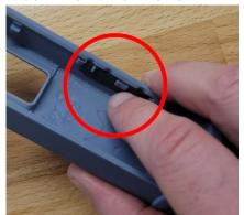
Insert the button panel into the area where there are 3 button windows of the case back. You'll have to sort of hold the case back at an angle to let gravity keep those buttons in place while you snap in the T-Beam in the next step.
