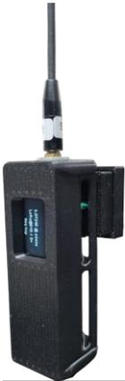
You can create a proximity sensing node by slightly modifying a T-Beam supreme. You do not have to add a relay, but the instructions below cover adding both a mmWave radar and relay.
