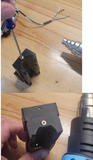
Using a soldering pin with an inset adapter or a heat gun and light pressure from a screwdriver, carefully press the inserts into the T-Beam back.
