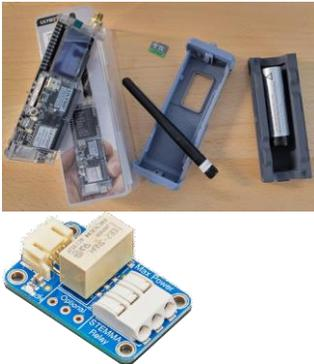
In order to signal the relay, the ChatterBox node sends a HIGH signal to the pin. So, in theory, any relay switch that can be signaled with a HIGH could be used. Here, I use an Adafruit non-latching relay.
