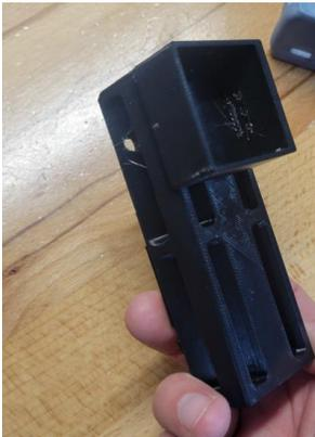
This case is based on an original design from [AlleyCat](#). I modified it to add a small enclosure for housing a relay module.
